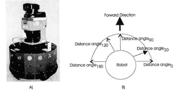
Figure 1: The Magellan Pro Mobile robot used in the experiments described in this paper (A) is equipped with 16 ultrasound sensors and a SICK laser scanner. This laser scanner has an opening angle of 180°, and it is able to deliver 180 distance measurements, one per degree (B).
