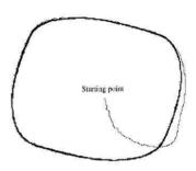
Figure 5: Robot's trajectory when the models corresponding to the translational and angular velocities were used. In this case the model used for the linear velocity was the one using ARMAX, while the angular velocity was modelled with NARMAX. The values delivered by the laser scanner are used as input information in both models. Compare this trajectory with the original trajectory shown in 2.
