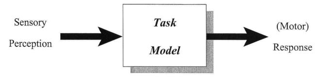
Figure 6: Task identification: a known function (such as the polynomial given in table 2) maps sensory perception to robot motor response
