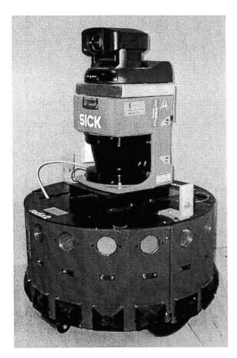
Figure 1: RADIX, THE MAGELLAN PRO MOBILE ROBOT USED IN THE EXPERIMENTS DESCRIBED IN THIS PAPER
