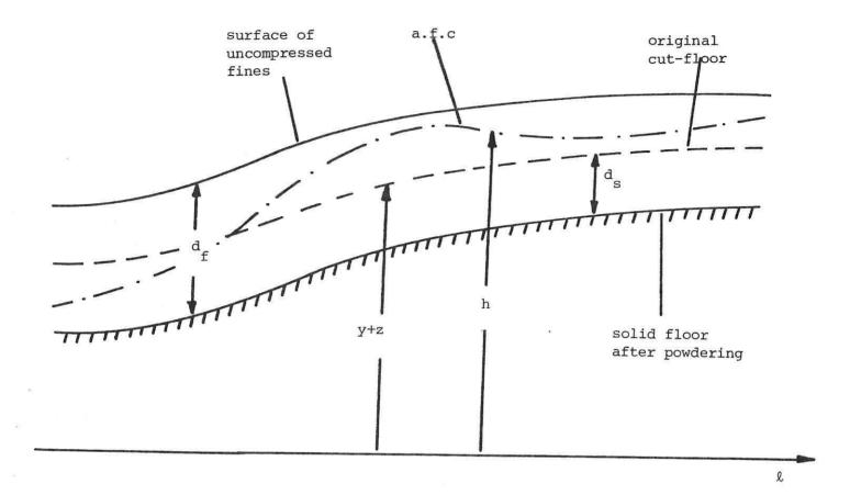
Fig. 4 Showing elastic beam model of a.f.c settling on powdered floor
