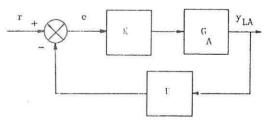
Figure 2 Linear feedback system with linear plant and measurement approximations
