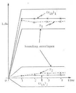
Figure 7 Closed-loom of real, nonlinear and approximate, linear feedback systems to a unit step domand in output one.
