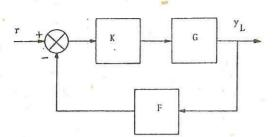
Figure 3 Linear feedback system with linear measurement approximation.
