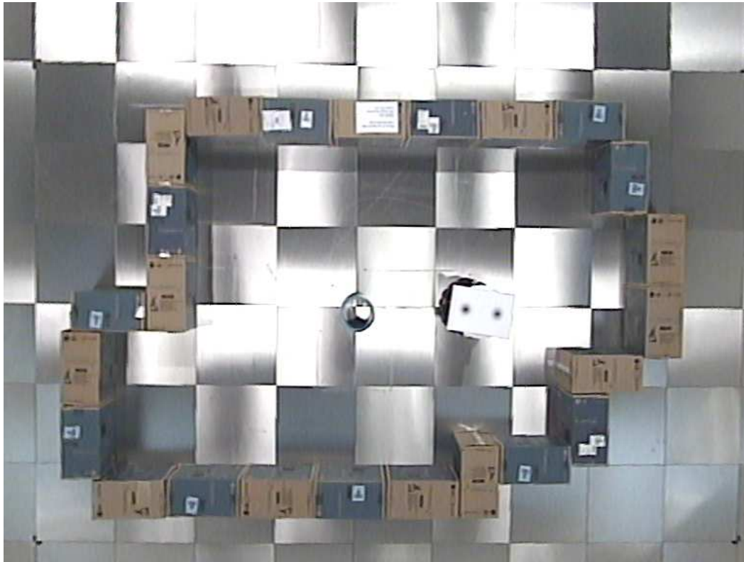
Fig. 4. Bird's eye view of an experimental setup. The longest width and height of the environment is 3.9 and 2.4 metres respectively. The image is taken with the overhead camera used for tracking the position of the robot.
