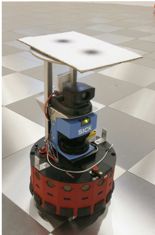
Fig. 3. Radix , the Magellan Pro mobile robot used in the experiments described in this paper. The visual target visible on the top of the robot was used for vision-based trajectory tracking.
