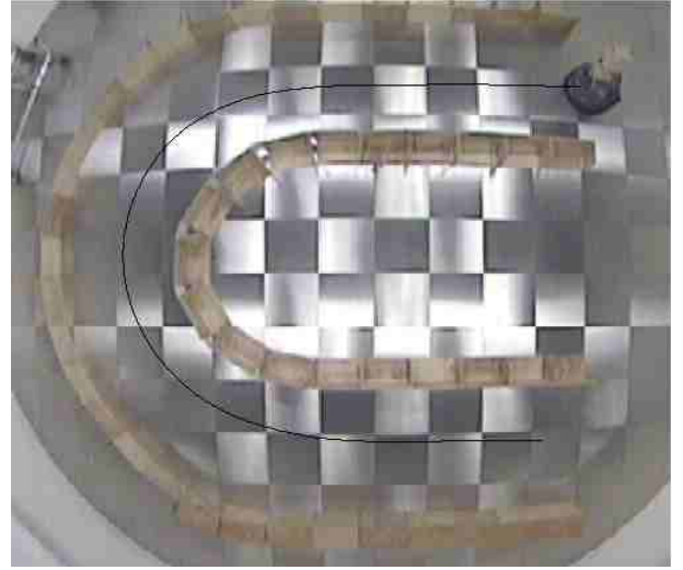
Fig. 7. EXPERIMENT 2: THE TRAJECTORY OF THE ROBOT UNDER CONTROL OF THE SENSOR-FREE POLYNOMIALS GIVEN IN TABLE 2. THE MODELS DRIVE THE ROBOT ALONG THE HUMAN TRAJECTORY GIVEN IN FIGURE 6 WITHOUT USING ANY SENSORY PERCEPTION. DURING THIS RUN, THE ROBOT LOGS ITS OWN PERCEPTION AND VELOCITY COMMANDS. THE LOGGED DATA IS THEN USED TO OBTAIN THE FINAL, SENSOR-BASED CONTROLLERS WHICH LINK THE PERCEPTION OF THE ROBOT TO MOTOR COMMANDS.
