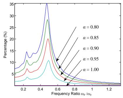
Figure 13 The percentage of the whole energy that the superharmonic components contain at different frequencies for different stiffness ratios
