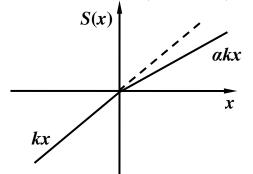
Figure 2. The restoring force of a bilinear oscillator
