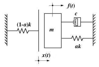
Figure 1. bilinear oscillator model
