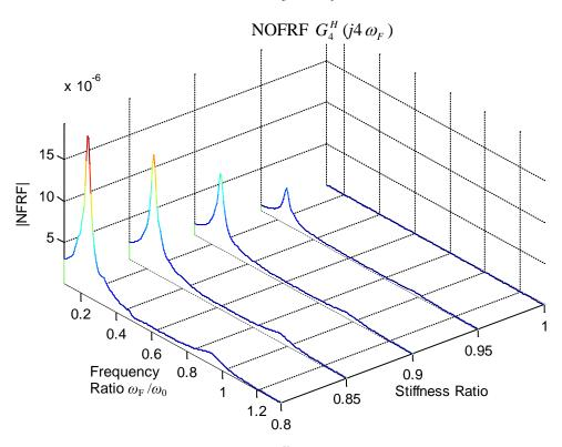
Figure 11 NOFRFs  $G_4^H$  (*j*4  $\omega_F$ ) at different stiffness ratios
