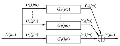
Figure 5. The output frequency response of a nonlinear system
