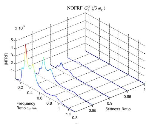
Figure 10 NOFRFs  $G_3^H$  (j3  $\omega_F$ ) at different stiffness ratios
