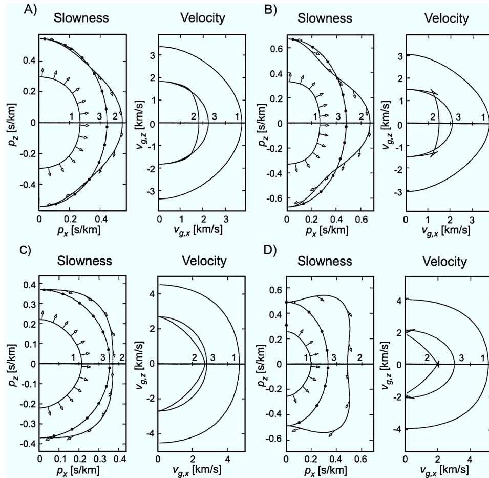
FIG. 1. Phase-slowness (left) and group-velocity (right) surfaces of the four shales A, B, C, and D considered in the numerical examples. Arrows indicate polarisations. Numbers 1 =  $P$ , 2 =  $SV$ , 3 =  $SH$ . See Table 1 for the elastic coefficients.
