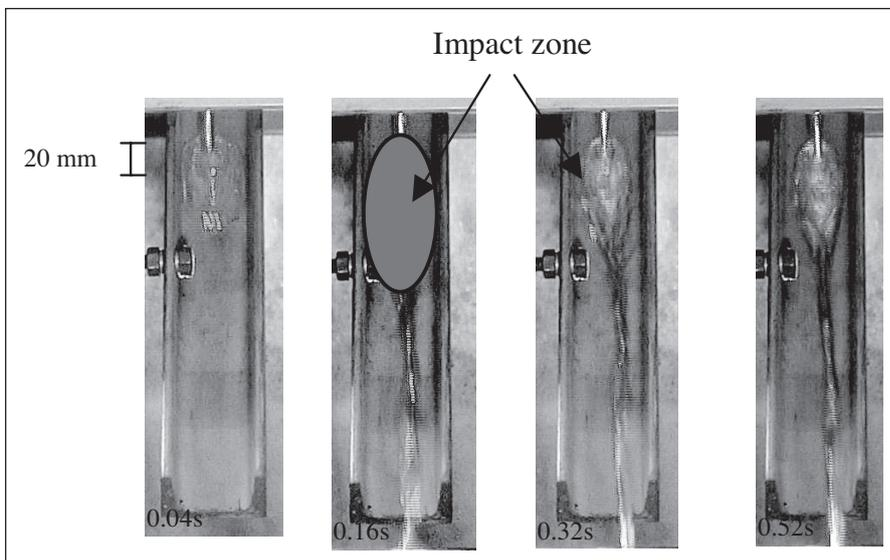
**Figure 4:** Sequential video images showing the molten A356 impacting on the cooling slope and then running as a narrow 'snake' down the cooling slope. Length of the cooling slope was 250 mm.
