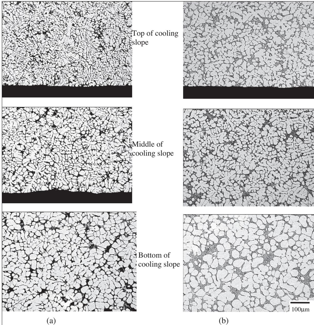
Figure 6: Microstructure of the remnant A356 on the cooling slope tilted at 45° and poured at: a) 630°C, 150 mm, b) 630°C, 250 mm.
