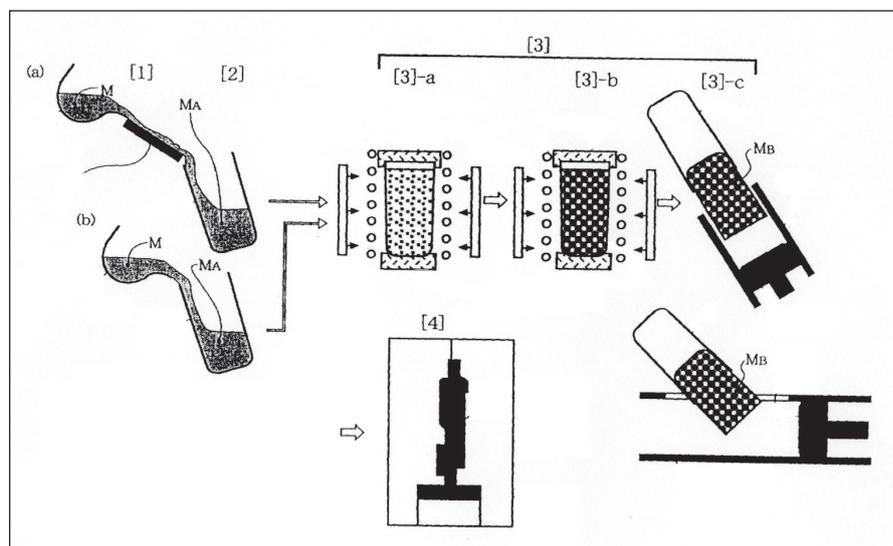
Figure 2: Schematic illustration of the development of thixotropic semi-solid structure in the NRC-process [4]. 1(a) is pouring down cooling slope with 1(b) pouring directly into the cup; 2 is the cup; 3-a is nucleation; 3-b is equilibration in the semi-solid state and holding with some heat input but still below the liquidus; 3-c is upending the semi-solid material into the shot sleeve (so the dross is left in the biscuit) and 4 is injection of the material into the die.
