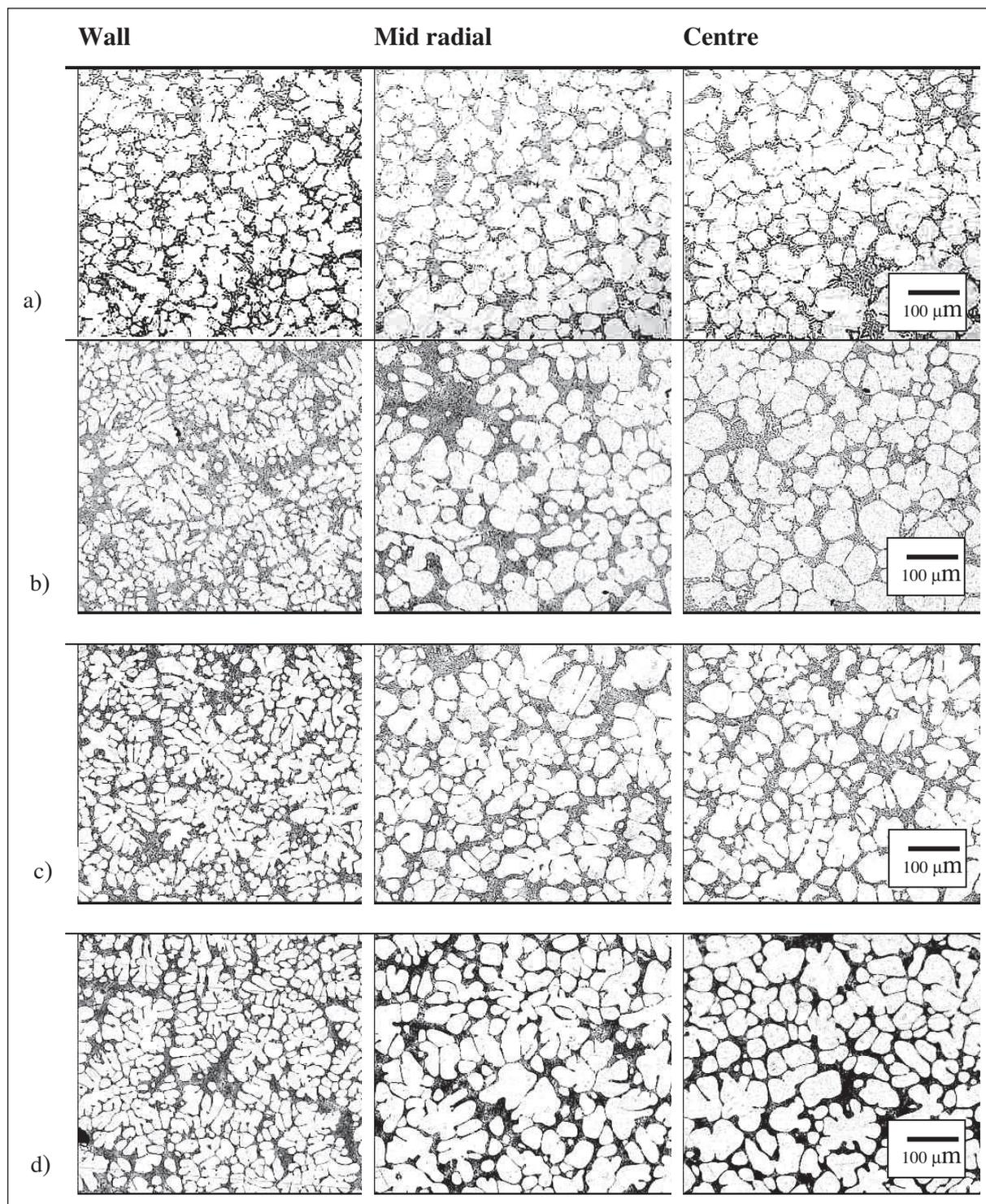
**Figure 5:** Effect of pouring temperature on samples poured into a cold stainless steel mould and then quenched. a) 620°C, b) 630°C, c) 650°C, d) 680°C.
