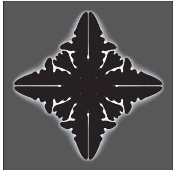
Figure 4: Solidification morphology resulting from growth under a composite four-fold + eight-fold anisotropy.
