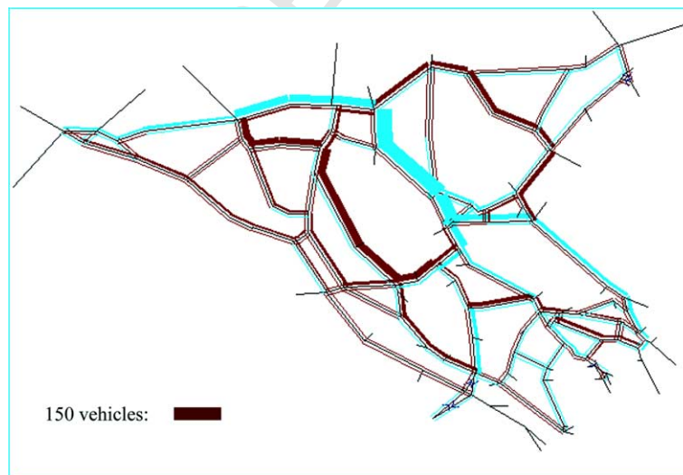
Fig. 9. Flow differences between the base and the scheme network averaged over the last 50 days. Black and grey indicate an increase and decrease of flow from the base to the scheme network respectively. The bandwidth is in proportion to the flow difference.
