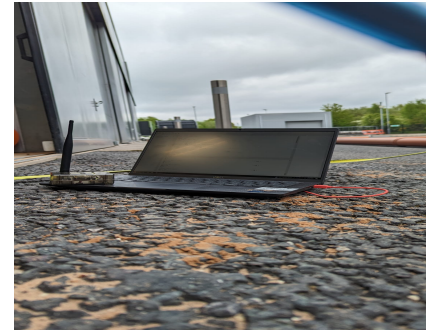
(c) The D node placed above the ground connected and powered by the laptop.
