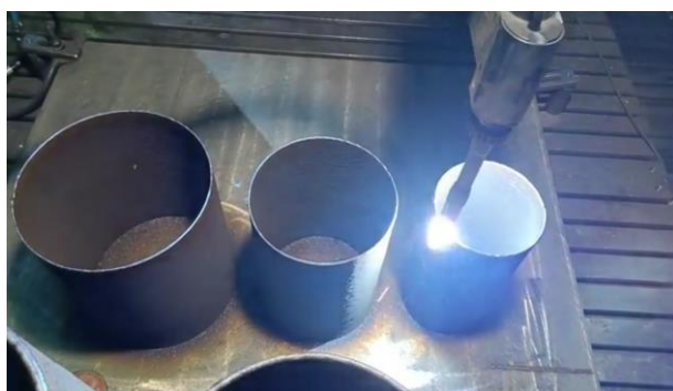
(a) WAAM CHS for compression tests
