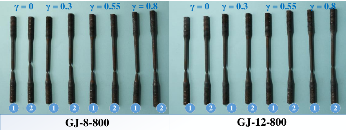
(f) After 20 min 800 °C heating.
