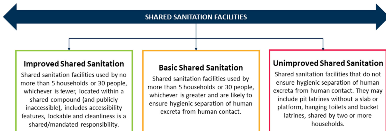
Fig. 4 | Proposed reclassification of shared sanitation facilities based on facility quality and user needs. Facilities are categorized into three groups—improved shared sanitation, basic shared sanitation, or unimproved shared sanitation—according to their quality and ability to meet user requirements.
