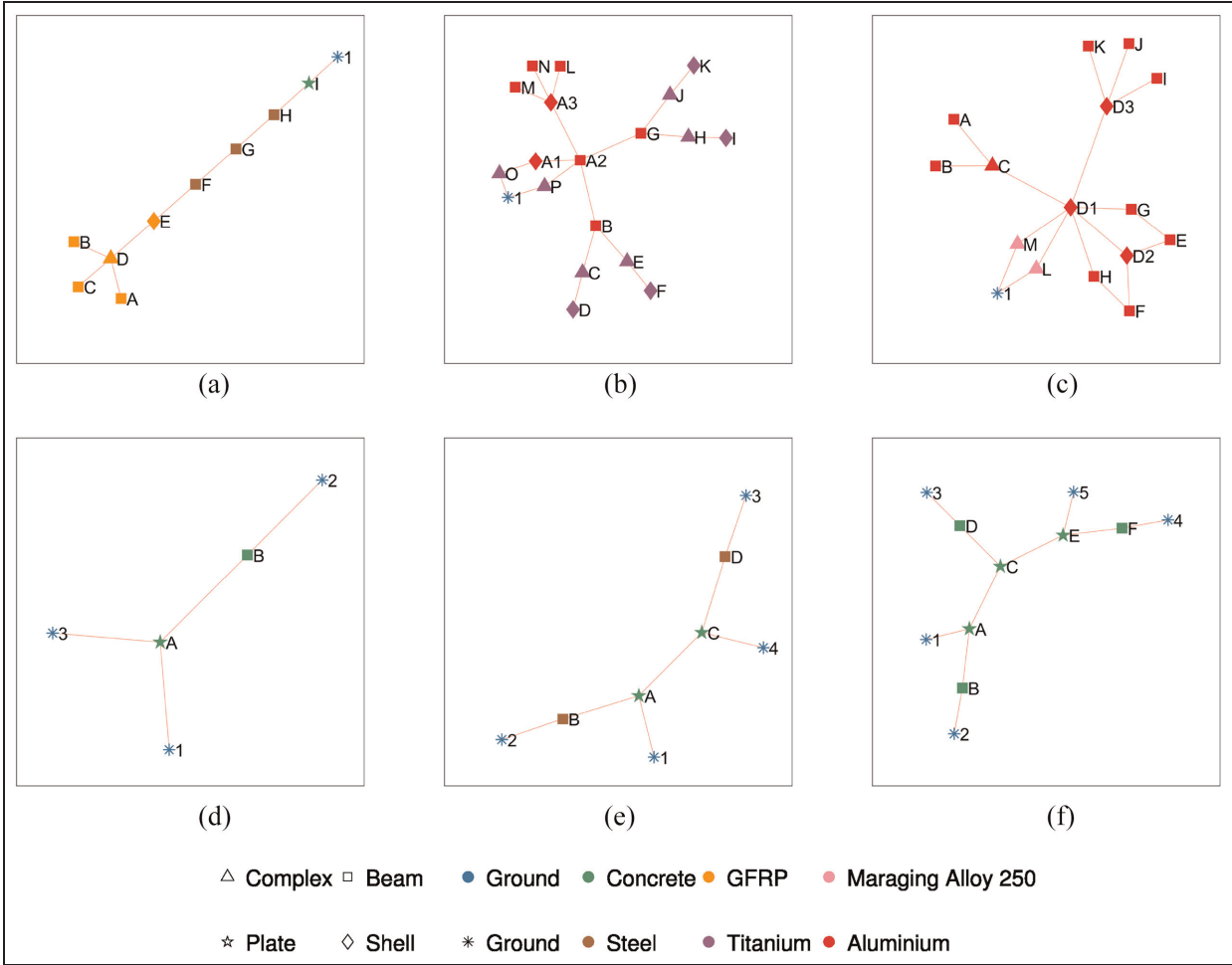
Figure 3. The graphs from Figure 2 re-imagined with element types (shape of the nodes) and materials (colour of the nodes) highlighted for visual comparison. (a) Turbine 1. (b) Aeroplane 1. (c) Aeroplane 2. (d) Bridge 1. (e) Bridge 2. (f) Bridge 3.
