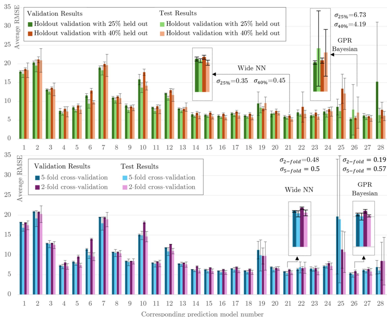
Figure 3. The statistical analysis of different ML models for two validation methods: holdout validation for 25% and 40% holdout and cross-validation for 2-folds and 5-folds. Both validation and test results are averages of five different runs, the error bars are calculated using the standard deviation ( \sigma ) of the five runs for each cases. The zoomed view of top two (lowest RMSE) prediction models, number 21 (wide NN) and number 26 (GPR Bayesian Optimisation) are provided. .
