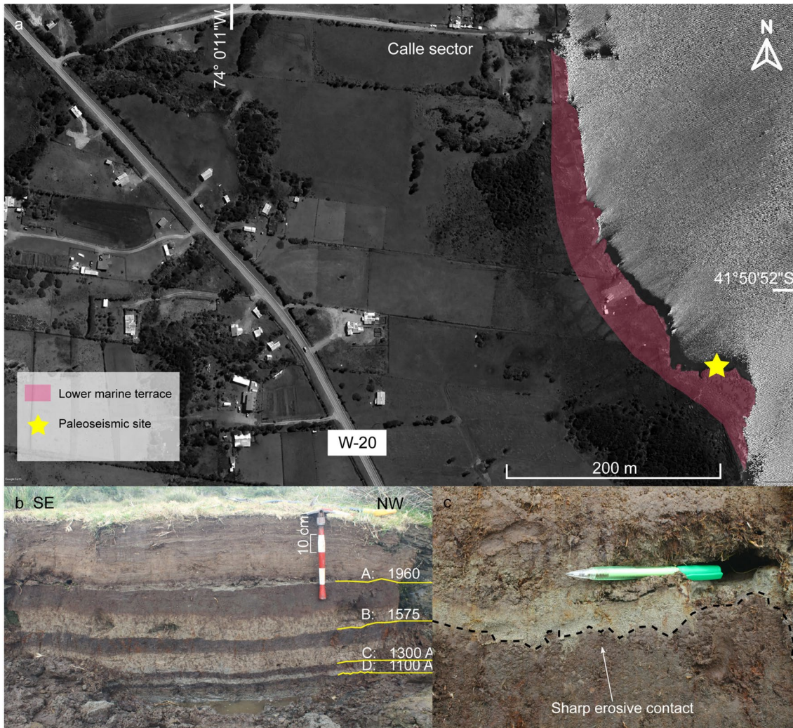
Fig. 10 Paleoseismic site of Chucalén a) Aerial image of Chucalén paleoseismic site, Los Lagos Region. b) Section of the stratigraphic profile of the constructional terrace of Chucalén where solid yellow line indicates the sharp lower contacts produced by the earthquake
