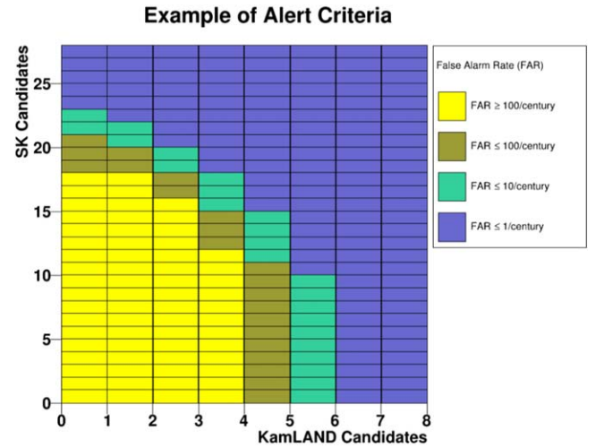
Figure 12. Example contour of the false alarm rates extracted from toy Monte Carlo simulation assuming the background-only hypothesis. The x -axis and y -axis are the numbers of candidates observed in KamLAND (in 24 hr) and SK (in 12 hr). The assumed background rates are 12.4 events per day in SK and 0.19 events per day in KamLAND, the same as those in the medium reactor activity scenario.
