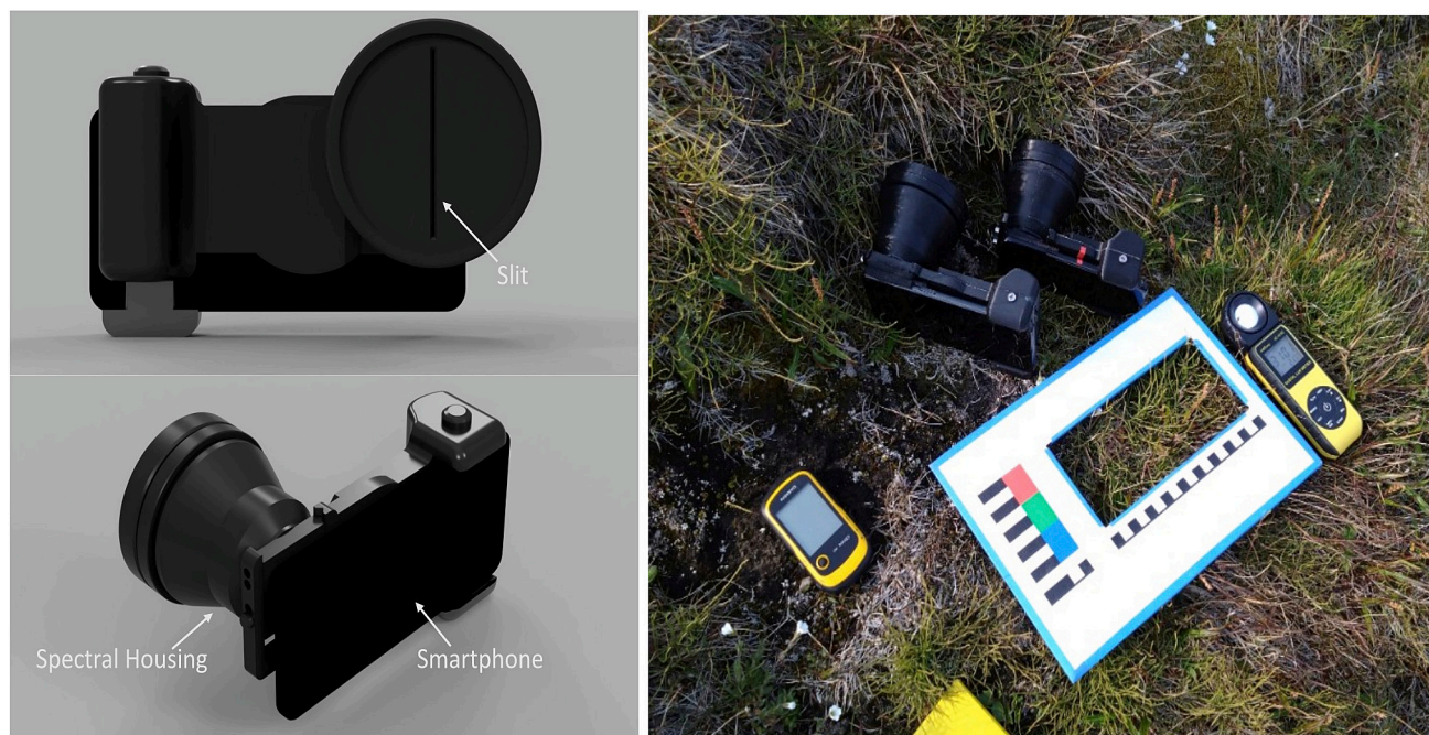
Fig. 2. The Hyperspectral Smartphone. 3-D render of the instrument highlighting key components (left) and a photograph of the instruments in the field demonstrating their high portability (right).
