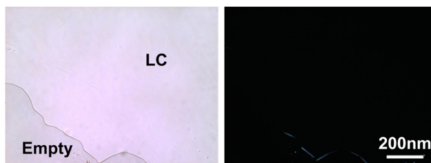
Fig. 4 Optical micrographs of the columnar phase of HATO6 sandwiched between two glass surfaces. (left) Bright field, (right) between crossed polarizers. (b) is completely black, showing defect-free homeotropic alignment. Similar homeotropic patterns were also observed for other non-fluorinated compounds used.
