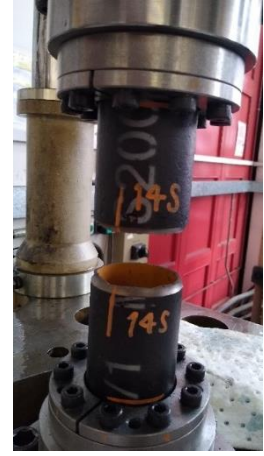
FIGURE 1 Examples of failed (a) sharp and (b) blunt notch uniaxial fatigue specimens.
