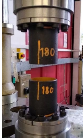
FIGURE 1 Examples of failed (a) sharp and (b) blunt notch uniaxial fatigue specimens.
