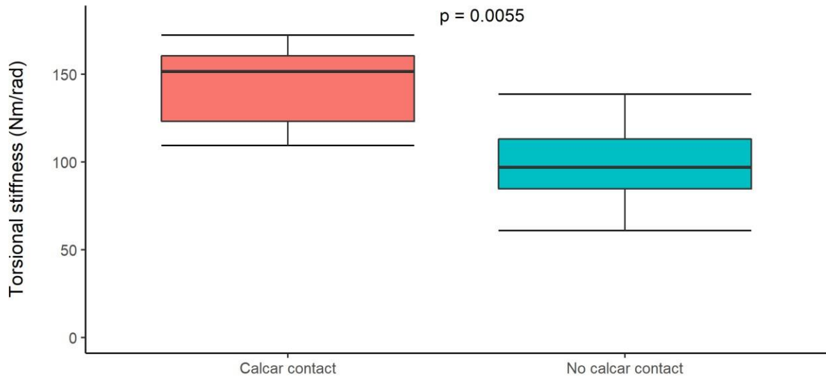
Torsional stiffness by calcar contact prior to fracture as seen on high speed video
