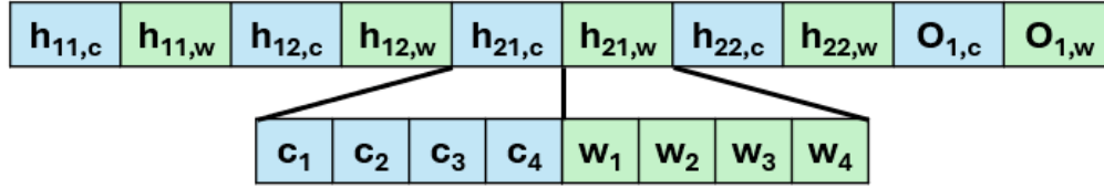
Figure 5: Genome encoding of the example network as shown in Figure 4 where each hidden and output node has two types of genes: connection genes and weight genes. The connection genes ( c ) are represented by blue color and weight genes ( w ) by green color. Hidden and output nodes can take inputs from all previous nodes. For example, hidden node h_{21} has four connection ( c_1, c_2, c_3, c_4 ) and four weight ( w_1, w_2, w_3, w_4 ) genes.
