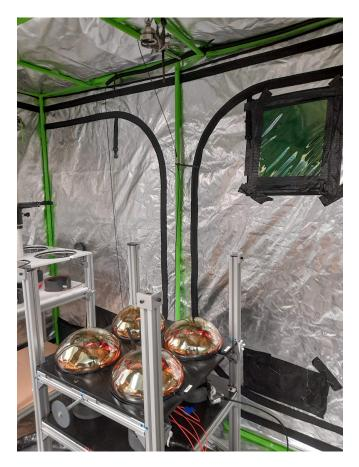
**Figure 2**: Mounting of the PMTs in the mechanical rig in the tent. Optical fibres guide the light from the LED box outside the tent to the diffuser, which hangs from a fixation point on the tent roof at the top centre of the image.
