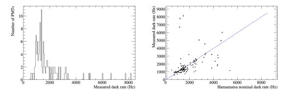
**Figure 8**: Results of the dark rate tests showing the distribution of measured dark rate distribution in 50 Hz bins for all PMTs tested (left) and the measured dark rates compared to the Hamamatsu nominal dark rates (right).
