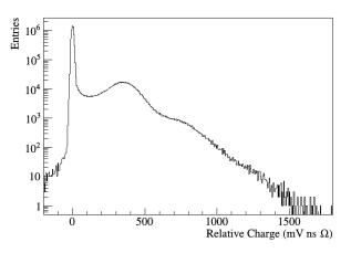
**Figure 4**: Typical relative charge spectrum with a pedestal peak at ~0 mV ns  $\Omega$ , a single-photoelectron peak at ~400 mV ns  $\Omega$  and later multiple-photoelectron peaks in the tail.
