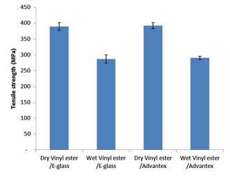
Fig. 9 Tensile strength of wet and dry vinyl-ester composite materials
