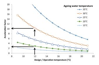
Fig. 2 Predicted acceleration factor for epoxy/E-glass composite due to ageing water temperature
