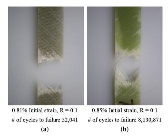
Fig. 11 Photographs of fractured test specimens
