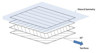
Fig. 1 ( $\pm 45^{\circ}/90^{\circ}/0^{\circ}$ )s Quasi-isotropic layup
