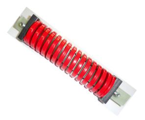
Fig. 3 Stressing mechanism for stress ageing of GFRP coupon
