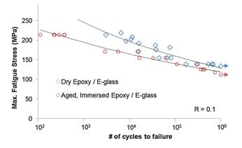
Fig. 10 Stress-life curves for wet and dry epoxy/E-glass in R=0.1 fatigue tests
