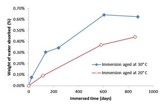
Fig. 6 Weight of water absorbed by Epoxy/E-glass composite during water immersion ageing
