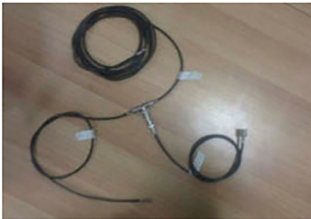
FIGURE 6 The Y-shaped network utilized to verify the forward model.
