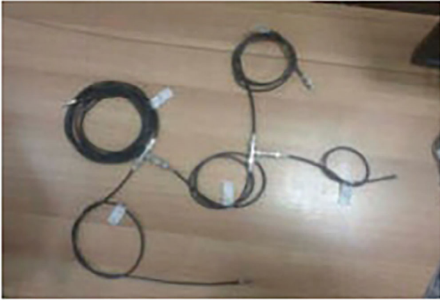
FIGURE 9 The YY-shaped network utilized to verify the forward model.
