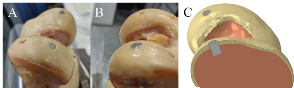
Fig. 6 Experimental image showing the metal pin positioning between the below flush hole 3 pin (A) and the flush hole 6 pin (B). The matching finite element model (C) shows the two metal pins, the hole 3 pin (back) below flush and hole 6 pin (front) flush
