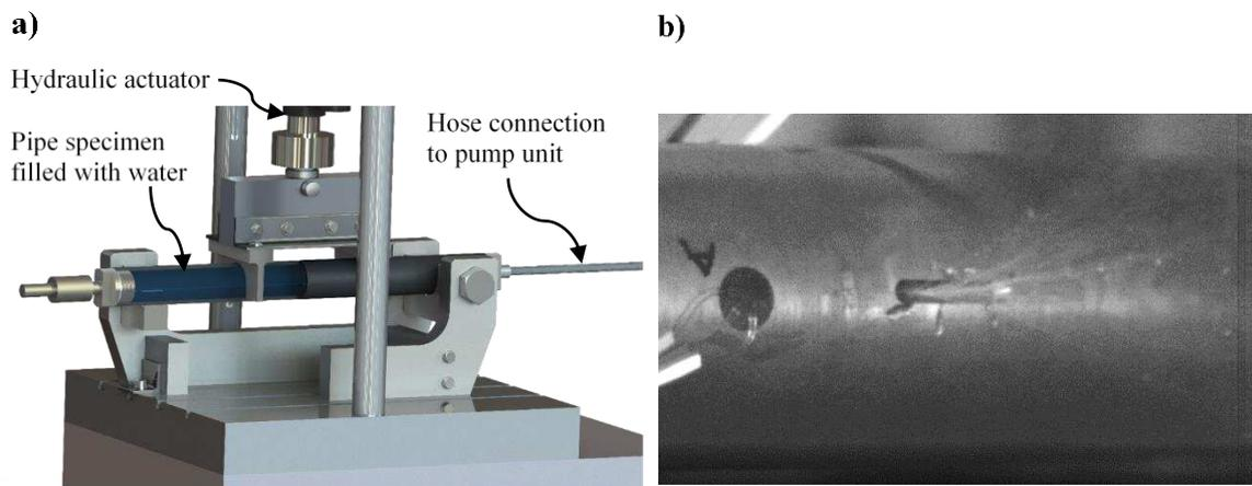
**Figure 6: (a) Cutaway render of the pipe biaxial fatigue test apparatus which is able to apply four-point bending and internal water pressure fatigue loads, and (b) an image showing a pitted pipe leaking as a result of water pressure fatigue loading.**
