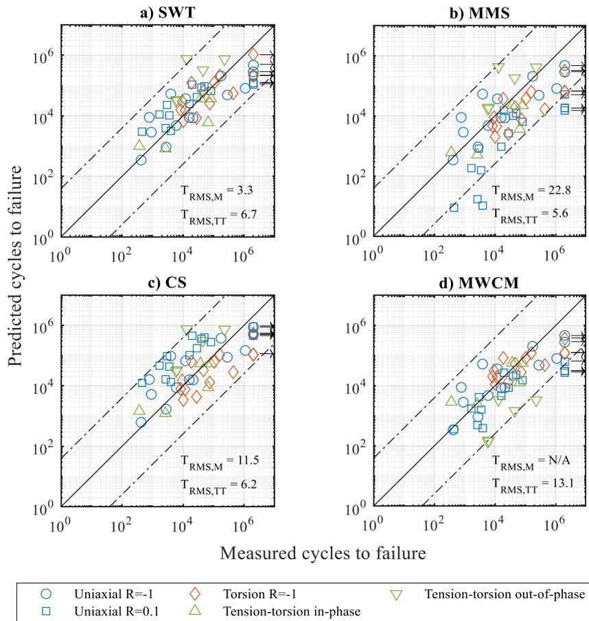
**Figure 3: Predicted cycles to failure vs measured cycles to failure for four fatigue criteria from John et al. [19]. Dashed lines show the fully reversed uniaxial scatter band.**
