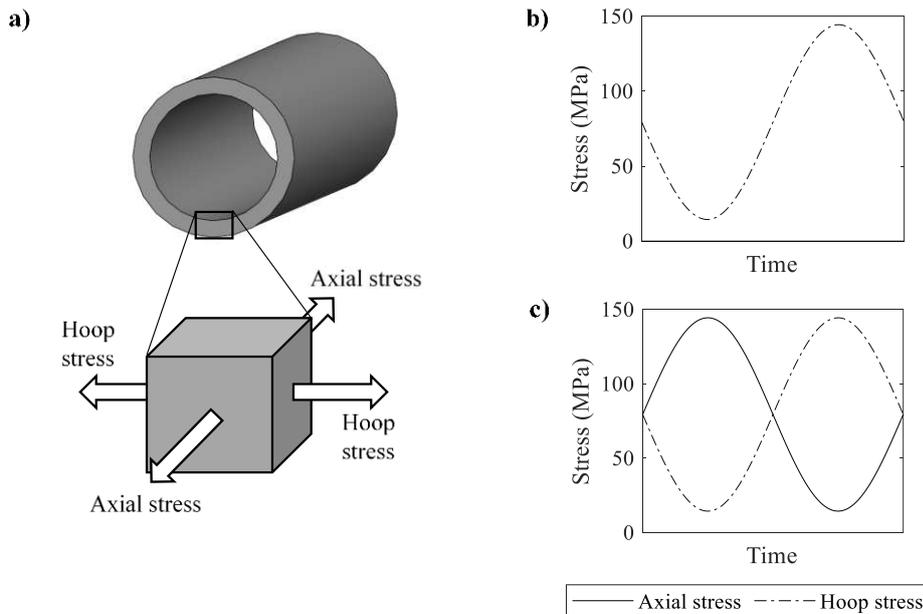
**Figure 4: (a) Schematic showing hoop and axial stress directions relative to a pipe and plots of a single stress cycle for the (b) uniaxial and (c) out-of-phase equibiaxial scenarios.**
