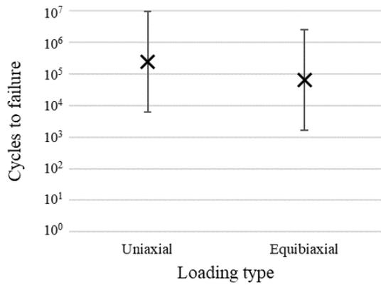
**Figure 5: SWT criterion predicted cycles to failure for uniaxial loading and equibiaxial loading. The error bars show the range between the P<sub>S</sub>=90% and P<sub>S</sub>=10% cycles.**
