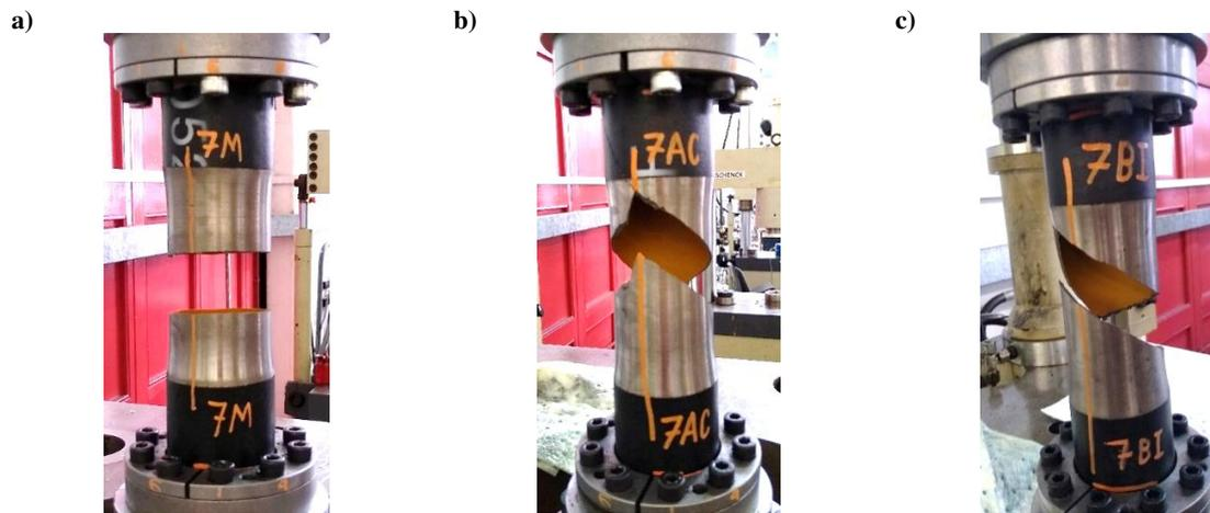
Figure 2: Examples of failed specimens tested under a) uniaxial loading, b) torsional loading, and c) out-of-phase tension-torsion loading from John et al. [19].
