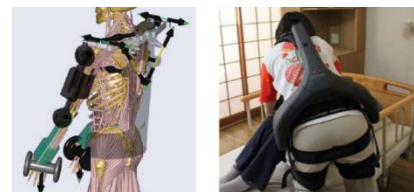
Fig 3.10 Medical worker exoskeleton optimised through musculoskeletal simulation.
