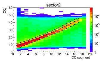
FIG. 7.  $\theta_{CC}$  versus CC segment number histogram in sector 2, where  $\mu$ ,  $\mu + 3\sigma$ , and  $\mu - 4\sigma$  are marked as black stars and fit by second degree polynomial functions shown by the curves.
