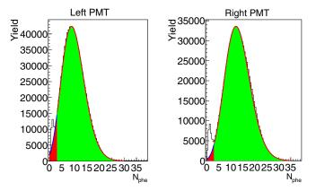
FIG. 8.  $N_{\text{phe}}$  histograms of the left and right PMTs in the tenth CC segment of sector 2 plotted separately and fit by the Poisson function in Eq. (11) shown by the red curve.
