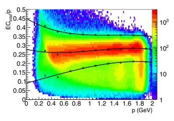
FIG. 9.  $E_{\rm total}/p$  versus p distribution, where the black lines show the upper and lower  $E_{\rm total}/p$  cut limits. The events outside the cut limits correspond to minimum ionizing particles and background.
