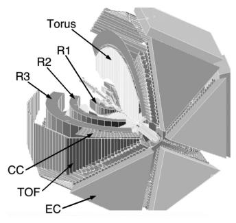
FIG. 4. Three-dimensional view of the CLAS detector cut along the beamline [8], with EC-electromagnetic calorimeter, TOF-scintillation counter, CC-Cherenkov counter, three regions R1-R3 of drift chambers, and the torus magnet.
