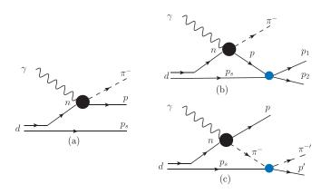
FIG. 2. Kinematic sketch of the three leading terms in the  $\gamma_v+D\to\pi^-+p+p$  process: (a) impulse approximation, (b) pp rescattering, and (c)  $\pi^-p$  rescattering. Diagrams (b) and (c) are the two main sources of final state interactions.
