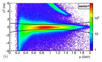
FIG. 10. (a) Typical negative pion  $\Delta T$  versus p histogram for sector 1 with upper and lower  $\Delta T$  cut limits. The bands above  $\pi^-$  upper  $\Delta T$  cut limit correspond to negative muons and electrons, separately. (b) Proton  $\Delta T$  versus p histogram for sector 1 with upper and lower  $\Delta T$  cut limits. The band above proton upper cut limit corresponds to  $\pi^+$ .
