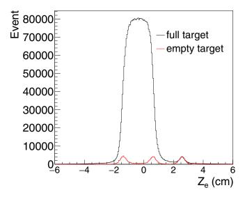
FIG. 6. Measured electron vertex ( $Z_e$ ) distributions for full target events (black) and scaled empty target events (red).
