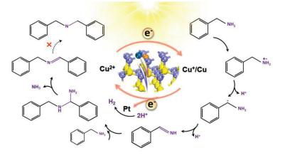
Figure 6. Proposed photocatalytic mechanism over CdS/Cu/Pt.
