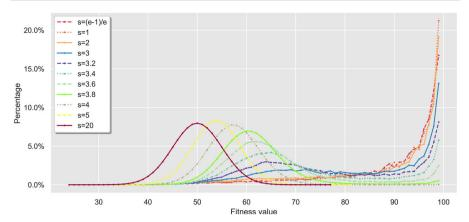
**Fig. 6** Percentage of fitness function evaluations used per fitness value for the self-adjusting  $(1, \lambda)$  EA on ONEMAX with n = 100 over 100 runs (runs were stopped when the optimum was found or when 1,500,000 function evaluations were made)
