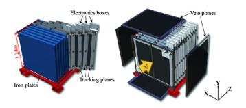
FIG. 4. An exploded view of a standard module.
