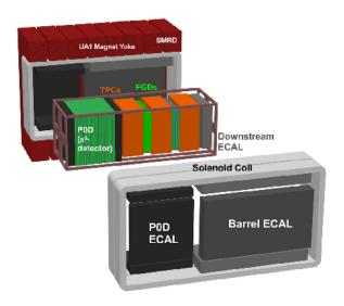
FIG. 7. An exploded view of the ND280 off-axis detector.
