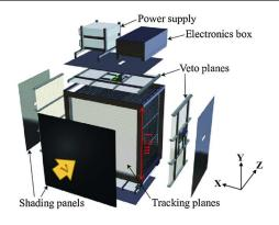
FIG. 6. An exploded view of the proton module.
