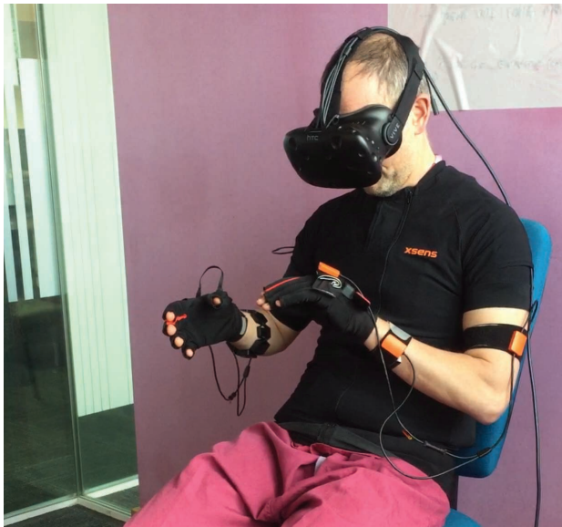
Figure 1. A participant wearing a VR headset; Xsense suit with IMUs sensors on the upper arms, forearms, and hands; and Manus VR gloves to control surgical virtual tools.
