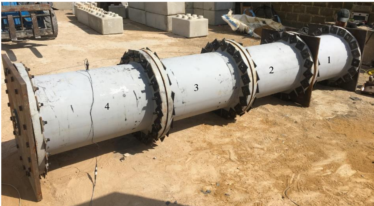
Figure 6: Four connected modules with a choke plate between chambers 1 and 2.
