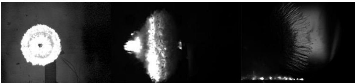
Figure 16: Images from high speed imaging using the Shimadzu HPV-X2 cameras showing: left) initiation of an electric detonator viewed end on showing the radial expansion of the detonator casing; middle) side view of a detonator showing the central weighting of the detonation products; and right) showing a wider field of view of the detonator fragments with a shadow graph of the fragments in motion, and bright spots where the fragments have struck the baseplate and ignited.
