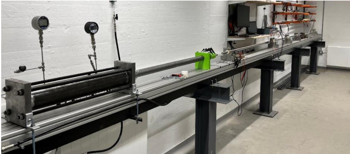
Figure 11: Photo of the Hopkinson Pressure Bar lab with the striker mechanism on the left hand side.
