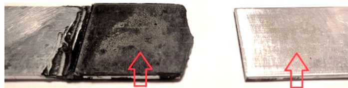
Figure 17. Ultimate adhesion failure in single-lap bonded joint specimen (arrows point bonded areas).
