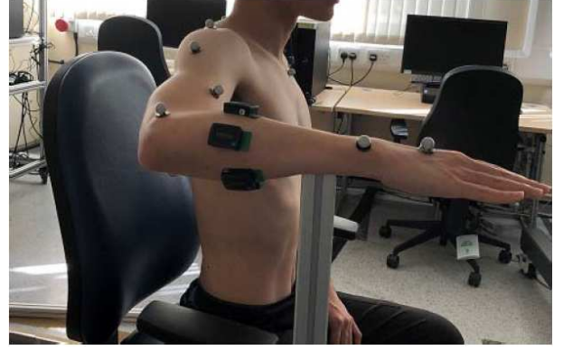
Fig. 1. Electrodes and markers placement in the data collection process.
