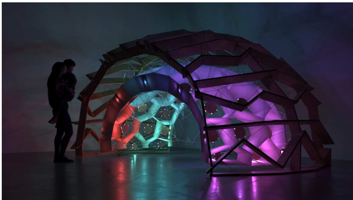
Fig. 1: Rendering of the structure with the proposed interactive lighting. Sensors on the outer structure provide input for light colours.
