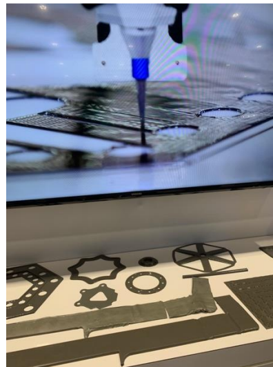
Figure 8. 3D-printed gasket for aerospace applications (PPG ARE™) [7].
