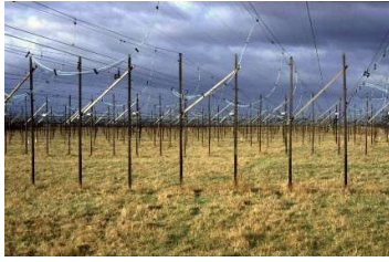
Figure 12. The IPS Array for investigating interplanetary scintillation, used to discover pulsars - Credit Graham Woan, University of Glasgow
