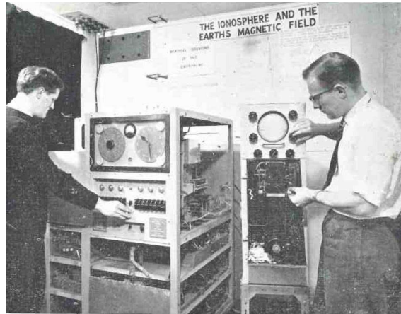
Figure 5. Researchers at Aberystwyth in the 1960s using an automatic ionosphere sounder for measuring the height of reflection of radio waves.
