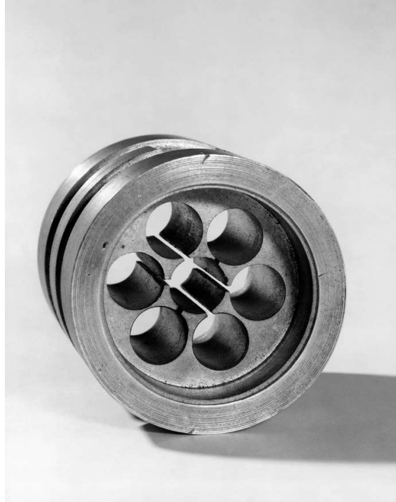
Figure 7. The anode block of the original cavity magnetron built in 1940 by Randal and Boot (from [14]).
