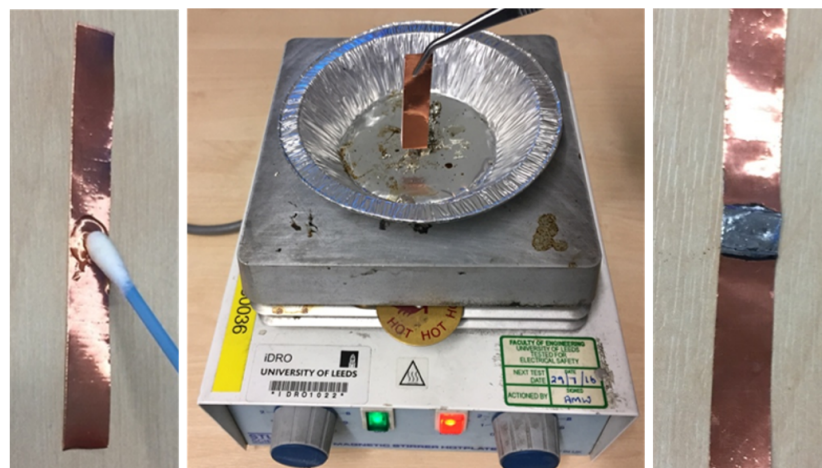
Figure 13. The method for applying Field’s Metal to the surface of copper tape. (Left) Applying flux on the surface of copper tape. (Middle) Dipping the copper tape into melted Field’s Metal. (Right) The pre-treated surface of the copper tape is covered by Field’s Metal.
