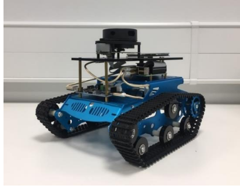
Fig. 1. Low-Cost Search and Rescue Robot Platform
