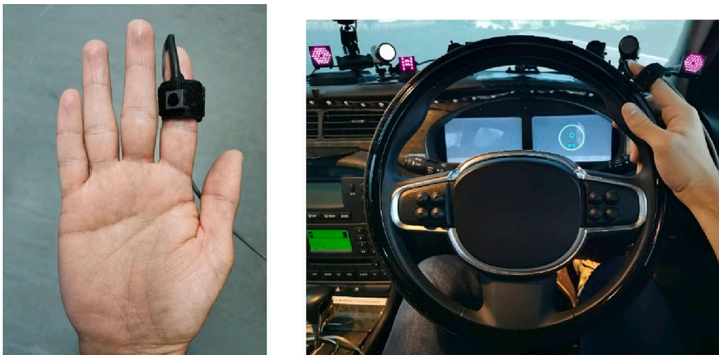
Fig. 3. The micro-switch button used for the study (left) and how it was used to provide a response (right).
