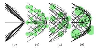
**Fig. 9** Short cantilever problem: Comparison between various definitions of damage. (a) volumes using various damage definitions. (b)-(e) optimal solutions with  $11 \times 21$  grid of nodes and various damage definitions: (b) per-member damage cases (p=16290), (c)-(e) damage at points on a  $6 \times 11$  grid (p=66) with (c) r=0.1L, (d) r=0.15L and (e) r=0.25L
