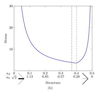
Fig. 18 Three-bar example: Analysis of all possible designs. (a) Nominal and worst-case compliance. (b) Worst-case stress. The dashed line represents the plastic stress-limited optimum structure obtained here, whilst the dash-dotted line represents the elastic compliance-optimized structure obtained by Stolpe (2019)
