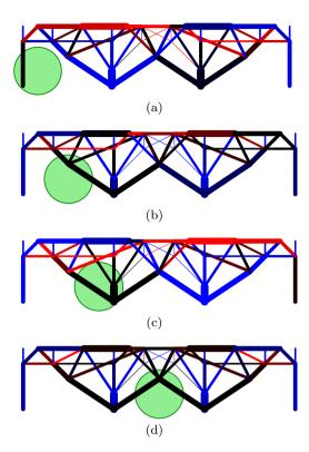
**Fig. 17** Spanning example, load-paths under selected damage cases. Blue members are fully stressed in compression, and red members are fully stressed in tension; darker members carry lower stresses. Relevant damage case shown in green
