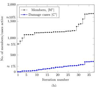
Fig. 10 Short cantilever problem: (a) CPU time taken to solve problem with per-member damage and various resolutions, solution speed with and without adaptive methods. (b) Number of members and damage cases considered at each iteration of the adaptive solution process for the case with 231 nodes - i.e. the largest result in part a - for which the full problem contains 16290 potential members and 16291 potential damage cases
