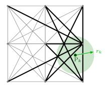
**Fig. 5** Damage case defined by point  $p_k$  and radius  $r_k$ . Thicker black members show those damaged in the given load-case, whilst thin grey members are undamaged. For this damage case,  $\mathbb{D}_k$  would contain the indices of the members shown with thick black lines
