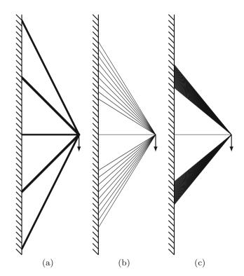
**Fig. 3** Short cantilever example: Results with extended design domain and nodal spacings of (a) L, (b)  $\frac{L}{8}$ , (c)  $\frac{L}{128}$
