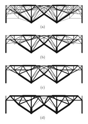
**Fig. 16** Spanning example, results with various filtering levels for r=1.6. (a) 0.01%, (b) 4%, (c) 9%, (d) 10%
