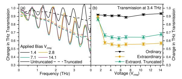
Fig. 4. (a) Terahertz transmission through the extraordinary axis of the 100 µm LCD (Device B) for untruncated (solid lines) and truncated (dashed lines) data at different LC bias voltages. The THz transmission through the 100 µm LCD at 3.4 THz is shown in (b), for both the ordinary (black down-triangles) and extraordinary (untruncated: yellow circles; truncated: green up-triangles) axes.
