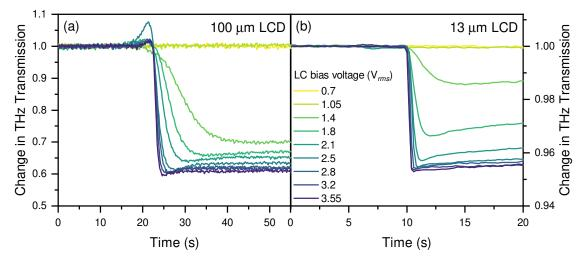
Fig. 6. THz transmission through the extraordinary axis of (a) the 100- $\mu$ m LCD (Device B) and (b) the 13- $\mu$ m LCD (Device C) as a function of the  $V_{\rm rms}$  voltage applied. The liquid crystal director was orientated parallel to the polarization direction of the collimated THz beam.
