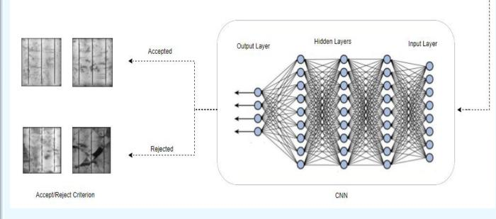
**Figure 1.** Incorporating the CNN network into decision making for the identification of solar cell cracks in an industrial setting application.
