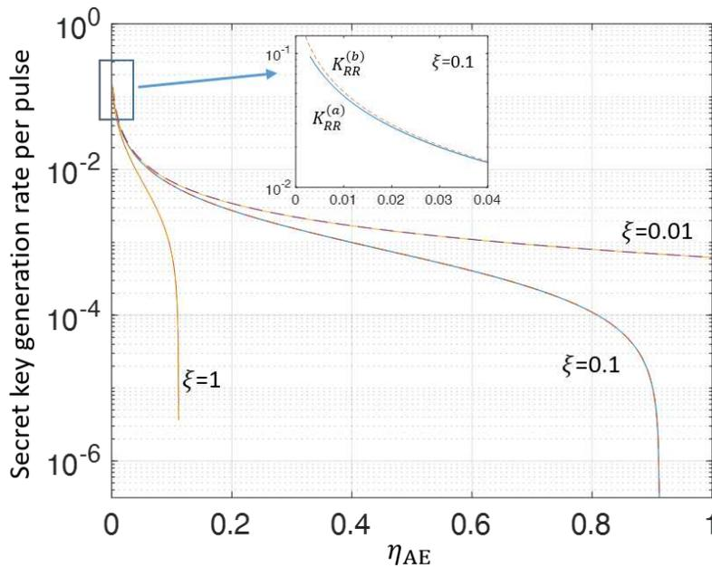
FIG. 6. Secret key generation rate, for the CV-QKD protocol in Fig. 4 with reverse reconciliation, versus  $\eta_{AE}$ . The solid lines represent  $K_{RR}^{(a)}$  and the dashed lines represent  $K_{RR}^{(b)}$ . As shown in the inset, the two curves are very close to each other, and mostly overlap except for small values of  $\eta_{AE}$ . In all graphs  $T_{eq} = 0.001$ ,  $V = 300$  in SNU,  $\beta = 1$ ,  $\eta_d = 1$ ,  $\nu_{el} = 0$ , and the excess noise is shown on the graphs.
