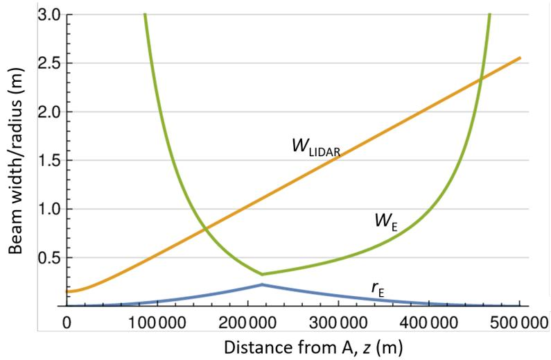
FIG. 12. The maximum radius,  $r_E$ , of the undetected Eve's object, the width of the propagating beam,  $W_{LIDAR}$ , sent by Alice, and the width of signal sent by Eve at point B,  $W_E$ , versus  $z$ .
