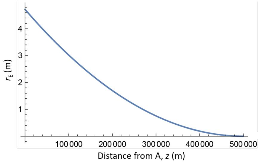
FIG. 9. The minimum radius for E's telescope aperture detectable by a typical radar system located at Bob's site. Note that the distance from Bob is measured by  $L - z$ . An object 500 km away from Bob must have a radius greater than 4 m, for our chosen parameter values, to be detectable by Bob's radar system.
