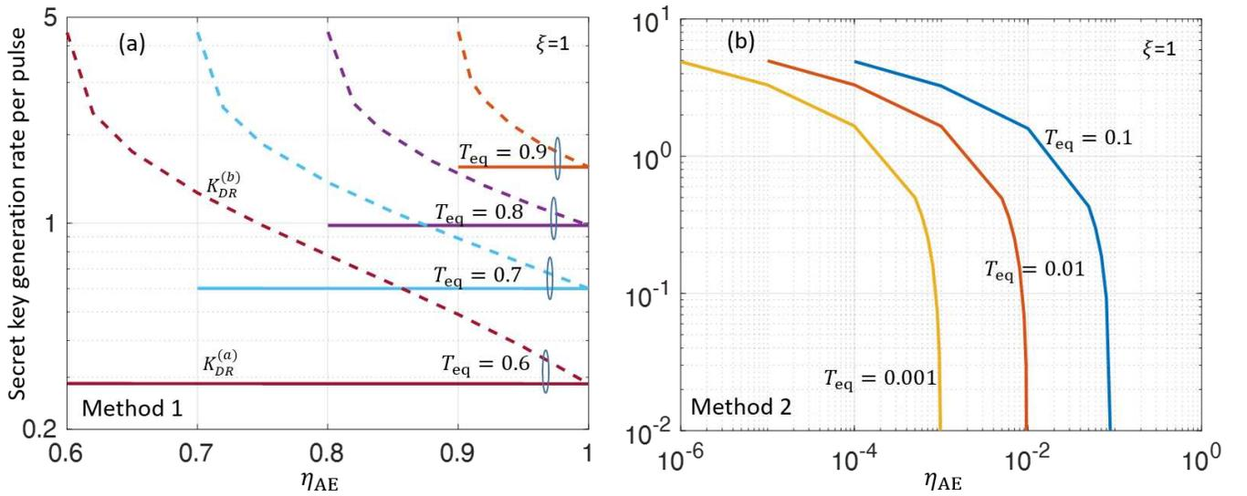
FIG. 7. Secret key generation rate, at  $V = 10^7$  in shot-noise unit (SNU), obtained from (a) Method 1 and (b) Method 2, versus  $\eta_{AE}$  for CV-QKD systems using direct reconciliation. The results are shown for an observed channel with different values of  $T_{eq}$ ,  $\xi = 1$  SNU,  $\eta_d = 1$ ,  $\nu_{el} = 0$ , and  $\beta = 1$ . In (a), the solid (dashed) lines represent  $K_{DR}^{(a)}$  ( $K_{DR}^{(b)}$ ).
