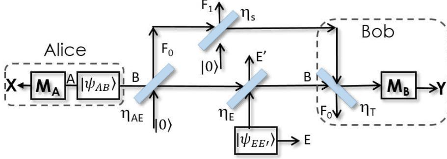
FIG. 4. A special setting for the setup of Fig. 3(a), where the bypass channel and the telescope actions are modeled by beam splitters. Eve's attack has also been modelled using an entangling cloner assuming that the Eve controlled section of the channel is also lossy.
