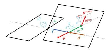
Figure 2: Kinematics of the reaction in the centre of mass system. The z-axis is oriented along the beam, y-axis is perpendicular to the ground; z' axis is oriented along the ejectile neutron direction, y' axis is perpendicular to the reaction plane.
