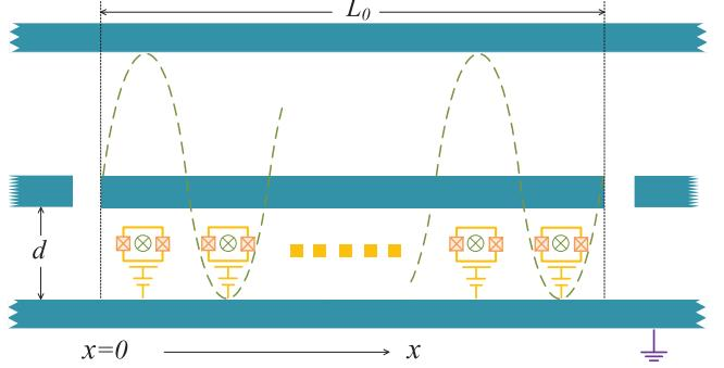
FIG. 3. Schematic of circuit QED design to generate the permutation-invariant QECC code. An array of charge qubits are placed inside a transmission line resonator.
